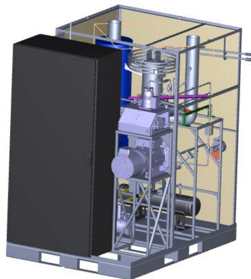
Liquid metal loop under construction in cooperation with Karlsruhe Institute of Technology
