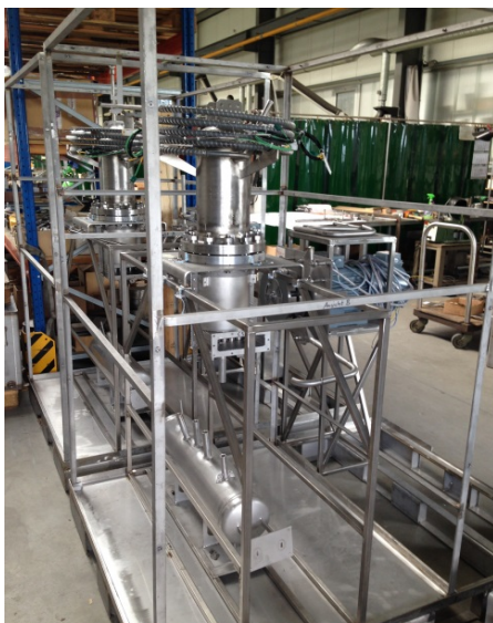
Liquid metal loop under construction in cooperation with Karlsruhe Institute of Technology
